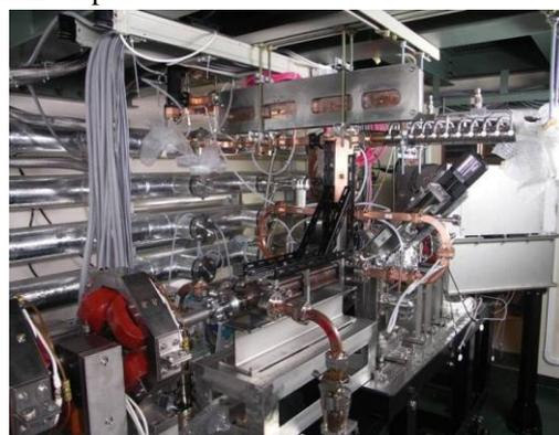
Fig.2 30 MeV X-band (11.424GHz) electron linac
