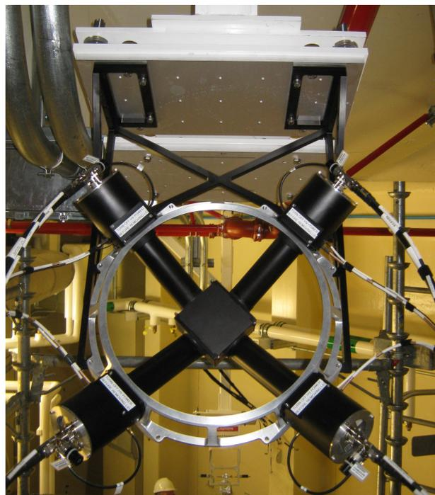
Fig.1. Picture of the new nToF detector installed at NIF.
